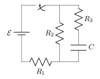
10. [Qid 2] (6 points) What is the potential energy stored in the capacitor just before the switch is opened?
