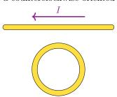
**Problem 6 (7 points)** A long straight wire is carrying an 8.00-mA current to the right along the x-axis in the positive x-direction. There is a coil of 25 loops that have a radius of 3.00 m with the center at the location (x, y) = (6.00, -8.00) where these values are in meters. What is the magnitude of current necessary so that the net magnetic field at the center of the loop is exactly zero?
