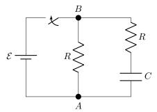
**Problem 12 (8 points)** If the switch in the previous problem has been closed for a long time, what would the current magnitude and direction be right after the switch was opened?
