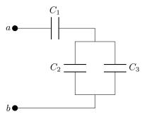
**Problem 2 (8 points)** A parallel-plate capacitor with plate separation of 2.0 cm has square plates, each with an area of  $6.0 \times 10^{-2}$  m<sup>2</sup>. A dielectric material with a dielectric constant of K = 2.4 is placed between the plates, completely filling them. What is the potential energy stored in the capacitor when a 4.0 V potential difference is applied?
