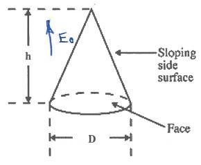
a) All E-field lines enter the botton surface of the cone and exit the side. Here,
