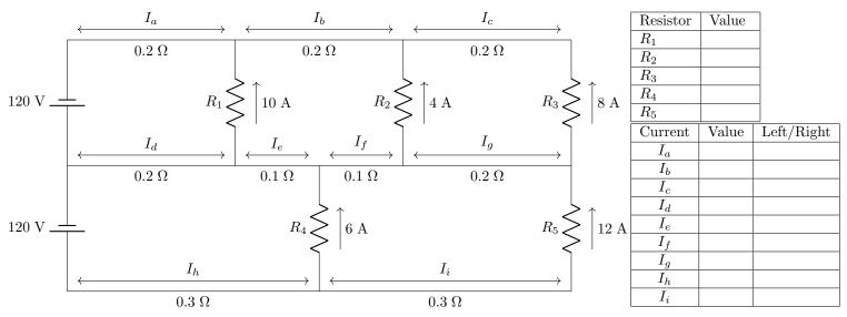
5. Find the current through each of the resistors in this circuit and the current through the battery.
