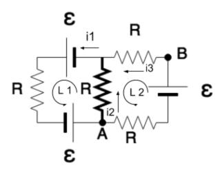
A. What is the current through the resistor **R** located in the center of the circuit (it is highlighted by a bold line)?
