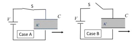
Select the correct relationship for the energy stored in the capacitor for the two cases after the dielectric is removed with respect to the energy in the capacitor before the dielectric is removed.
